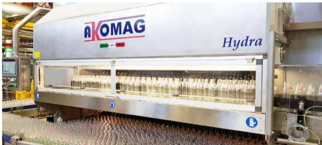
Hydra 8.2 reaches speeds up to 37,500 bottles/h and has a mechanical efficiency equal to 99.4%
